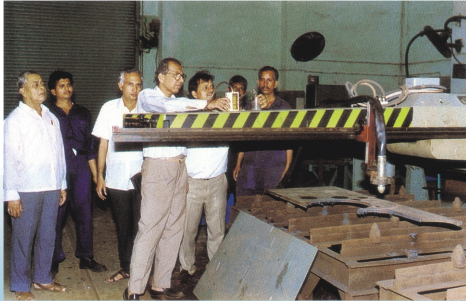
Industrial hygiene survey at Centre for Design and Manufacture during plasma cutting operation for estimation of ozone and NOx
